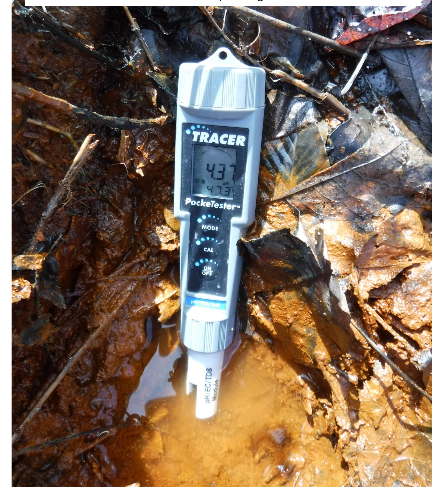
Numerous acidic seeps and outfalls from the Keystone and Revelation Companies' mines caused the Dept. of Environmental Protection to list Kanawha Fork as biologically impaired. Note the very low pH of 4.37 shown on the meter below. Photo courtesy of Doug Wood
